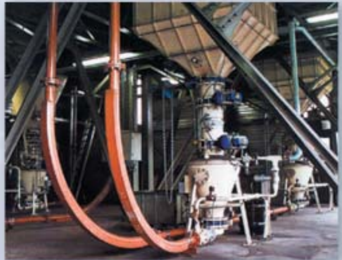
■ Dense phase conveying of foundry sand
