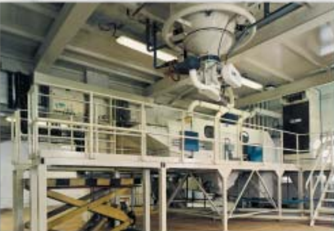
■ Processing installation for pigments and fillers using an "Galahad" automatic bag-emptying machine complete with scissor lift, baling press and filter installation
