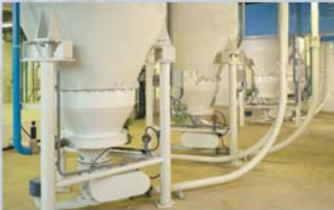
■ Vacuum conveying of colour additives / pigments
