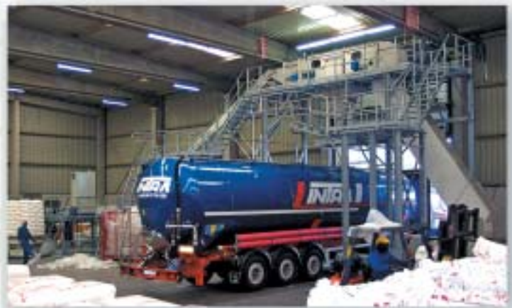
■ Processing installation for pigments and fillers using an "Galahad" automatic bag-emptying machine complete with scissor lift, baling press and filter installation
