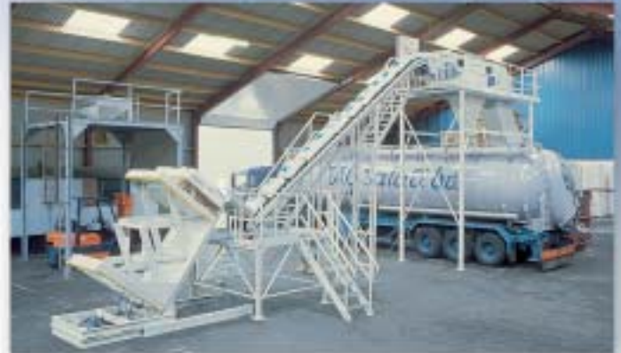
■ "Bags-to-Bulk" system for plastic granules and powders incorporating "Galahad" automatic bag emptying machine.
