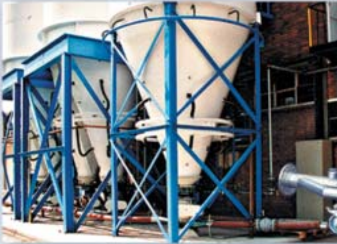
■ Dilute phase conveying of titanium dioxide
