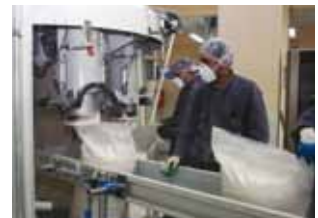
The bag is transferred in the upright position into the bag closing device
