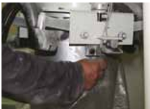
The empty bag is placed onto the spout
