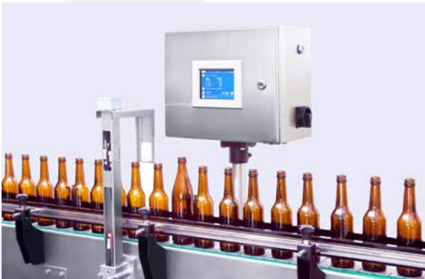
miho **Unicon 3** is a bottle sorting system that uses the light barrier technology. It detects bottles with a different height and rejects them. The reject system detects **bottles with different heights and lying bottles and bottle-breakages** and initiates their rejection, even through different reject systems if required.
