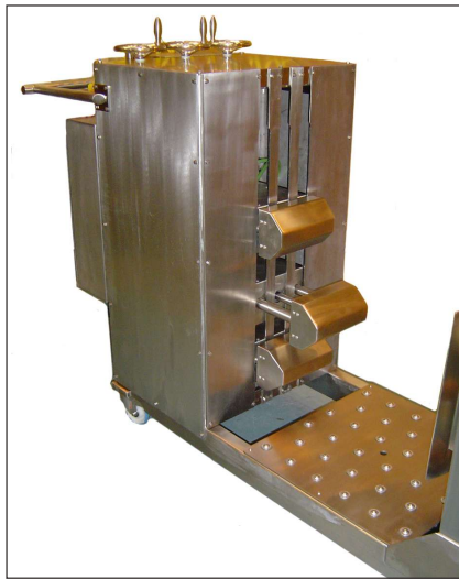
PalPharMassage cylinders can be adjustable to suit different drum heights and powder fills within the drum.
