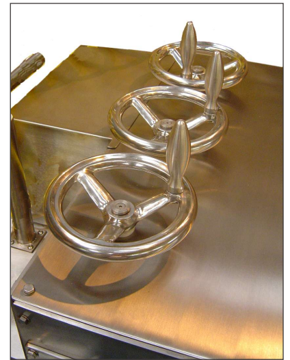
Cylinders can be easily adjusted using stainless steel hand wheels. There is also an option to adjust the backstop for drums of different diameters.
